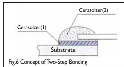
This method includes pre soldering as the first step to ensure proper bonding with substrate. The lead wire is already coated with Cerasolzer. Pre-soldered substrate with Cerasolzer(1) and a Cerasolzer coated component (lead wire etc.) are bonded by using ultrasonic oscillations, heat and more Cerasolzer(2).
