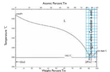
Fig.2 Phase diagram of Sn-Zn system
