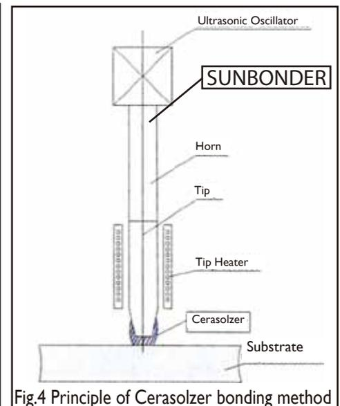
Fig.4 Principle of Cerasolzer bonding method
