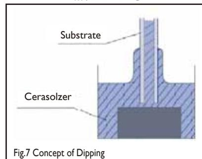
This method applies an ultrasonic bath where Cerasolzer is melted in order to coat a larger area of shaped substrates. It is even possible to inject Cerasolzer into the inner cavity of the cylindrical substrate.
