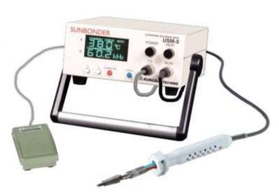
Japanese portable ultrasonic soldering system with ultrasonic transducer activated by a foot switch. Includes automatic tuning function using phase-locked loop that automatically locks the generator to the resonant frequency of the transducer, even under varying conditions of temperature and load. Ideal soldering device for small area applications.
