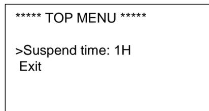
Suspend time is possible to change by pushing Switch A when the cursor ">" is "Suspend time" position.
